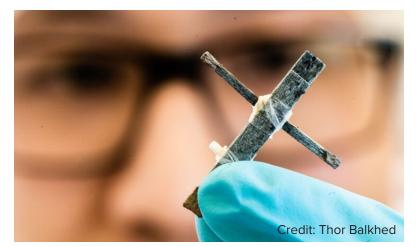
grainless wood that is evenly structured throughout. They removed the lignin, leaving only long cellulose fibres with channels where the lignin had been.
