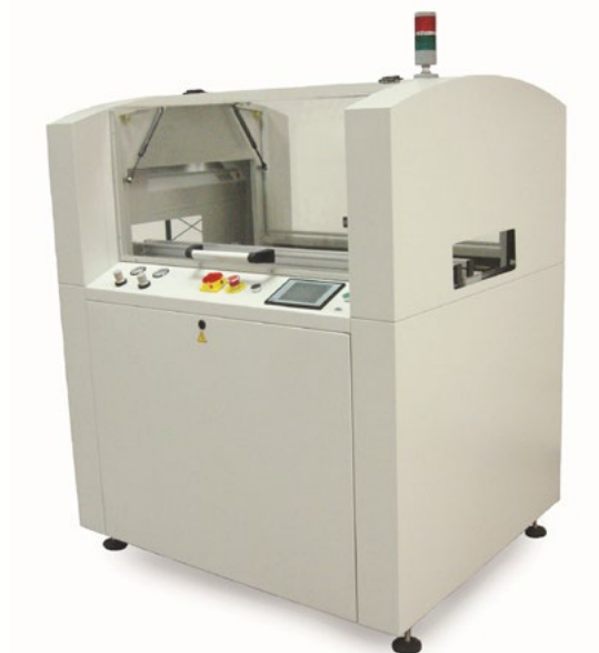
Figure 6: Example of a selective soldering system.
