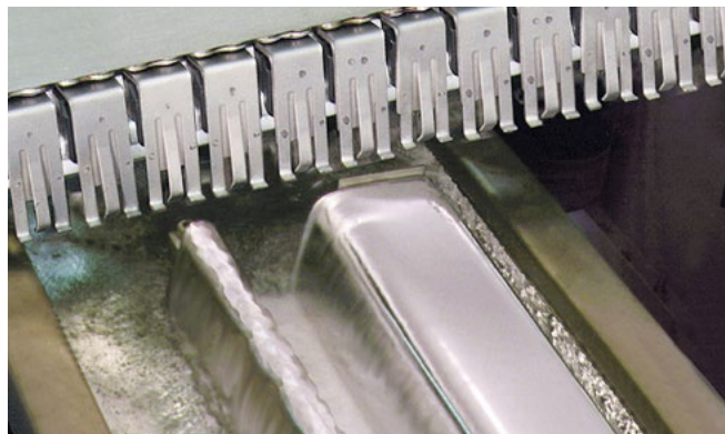
Figure 3: Example of transport fingers in a wave soldering system. Note the waterfall of hot solder that makes contact with the board components.
